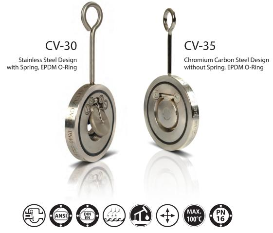
The main difference between standard swing check valves and wafer type swing check valves is that the wafer types do not have the full-bodied arrangement. When the valve opens, the disc is forced into the top of the pipeline. Due to a very short face-to-face dimension the body has a reduced bore. Swing type wafer check valves are virtually maintenance free, the disc is self-centering and protected and it has a special limit stop to protect against pipeline damage.
